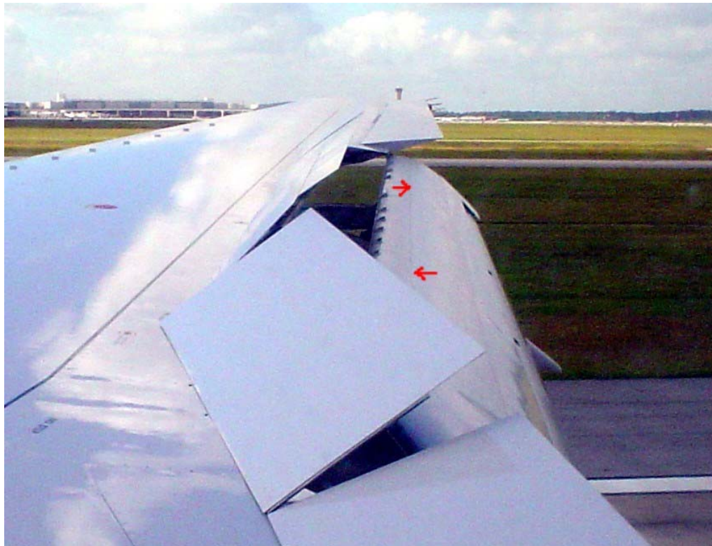
Photo 4. Fractured flap after landing
