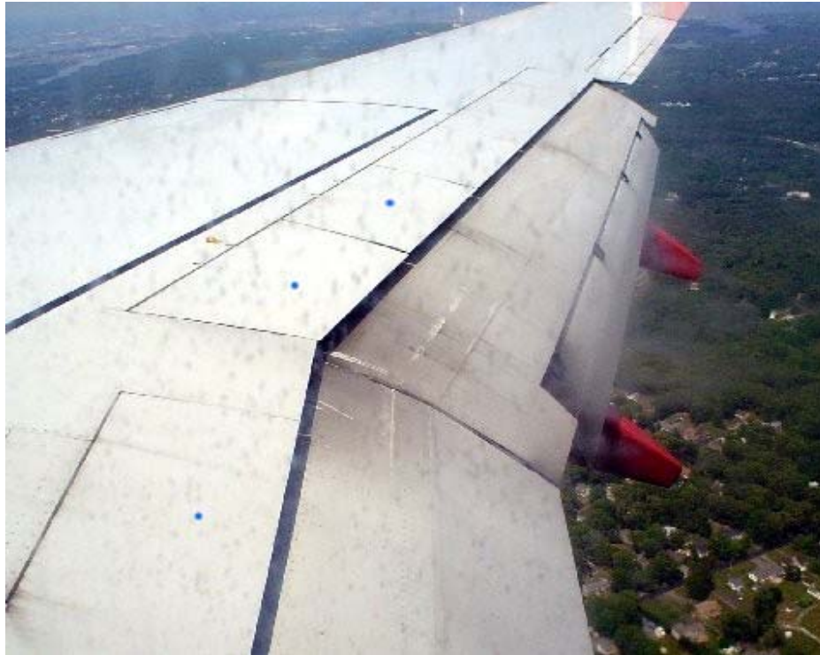
Photo 6. Shadows cast by 737 spoilers on undamaged flap
