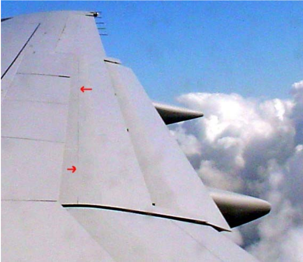
Photo 2. Stress fracture on 757 outboard flap
