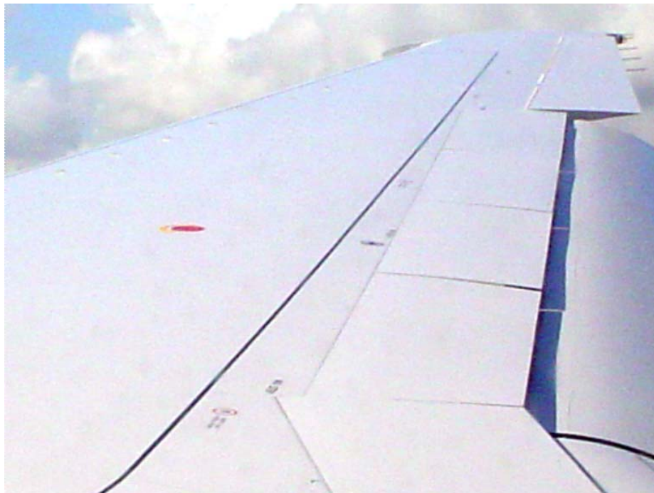
Photo 7. Shadows cast by 757 spoilers on damaged flap
