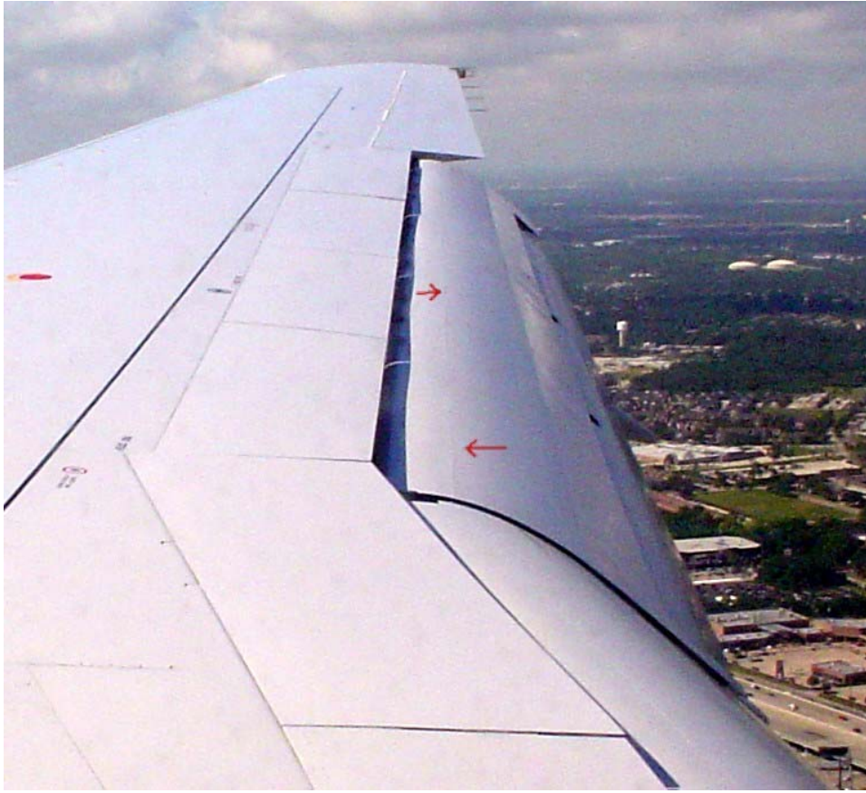
Photo 3. Stress fracture on 757 outboard flap fully deployed for landing
